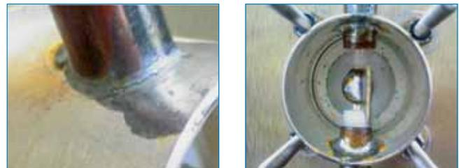
Antenna showing oxidation within the power divider. Tests with vector analyzer line sweep test did not reveal the problem. PIM 21 test system could however clearly detect the issue and pinpoint the faulty component.
