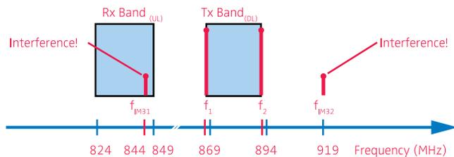
Example of intermodulation caused by two CW signals. Since the channel bandwidth of RF transmitters occupies usually a frequency range, resulting IM appears in a range of frequencies.
