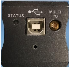
Figure 2.3 The power sensor end panel showing the connectors and Status LED.
