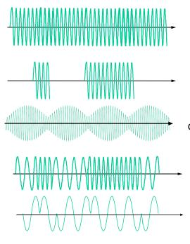
CW Signal – Continuous Waveform with static power level
