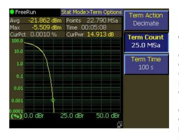
In a non-statistical peak power measurement the peak-to-average ratio is the parameter which describes the headroom required in linear amplifiers to prevent clipping or compressing the modulated carrier. The meaning of this ratio is easy to visualize in the case of simple modulation in which there is close correspondence between the modulating waveform and the carrier envelope. When this correspondence is not present, the peak-to-average ratio alone does not provide adequate information. It
