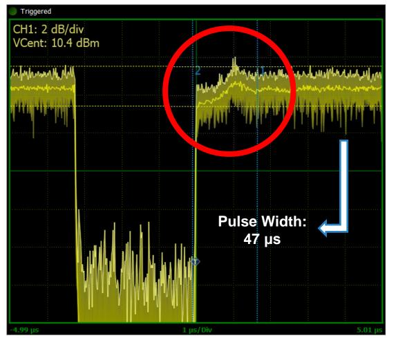
• Settling Time: 90% to Signal's Steady State Max Level
